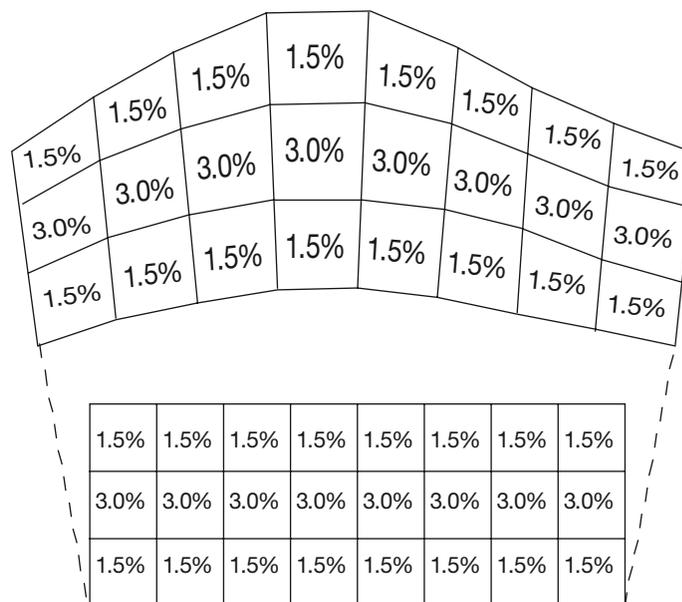
**Figure 4-23** – Adjusting a probability map for drift motion when drift forces vary from one place to another in the possibility area (drift distance and area expansion exaggerated for clarity)
