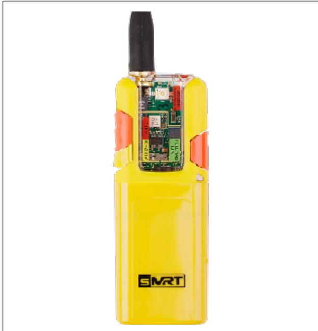
Figure 28 — Maritime survivor locating device (Man Overboard Device) using AIS and VHF DSC
