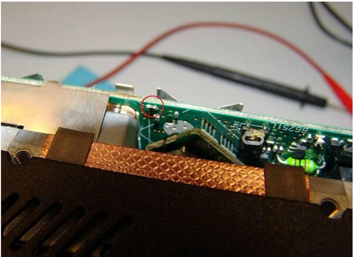
5. Put a drop of thermal compound over the resistor, to thermally couple the NTC to the heatsink. Make sure you touch the aluminium heatsink and the NTC! This will make the fan much more accurately responsive to temperature changes.
