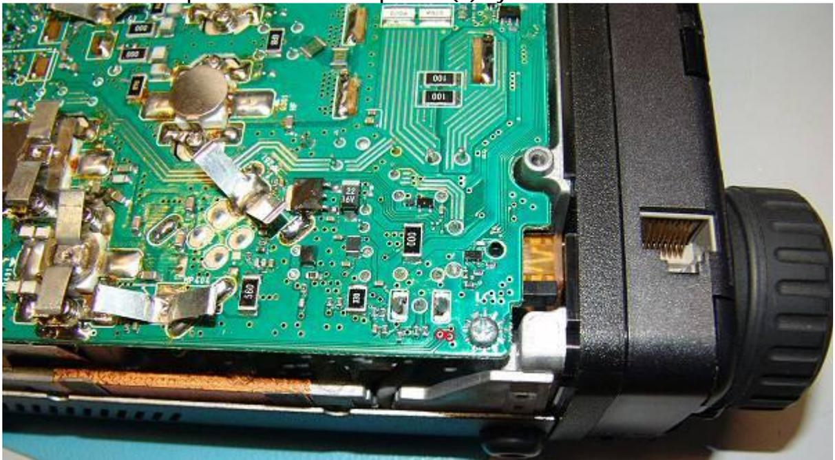
3. Clean the pads, and pre-tin them, solder the resistor to the pads
